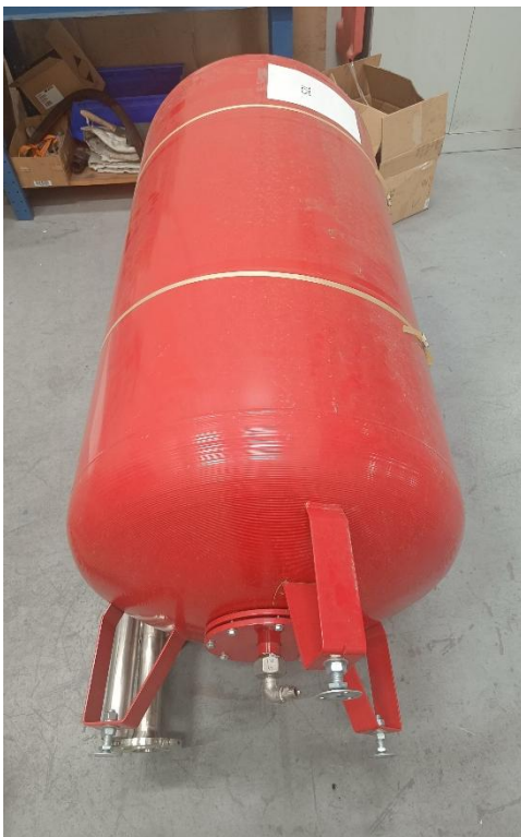
Figure 5: Low-pressure syngas buffer vessel of 800 L. The vessel is to be installed adjacent to the GtL system at the IMDEA site.
