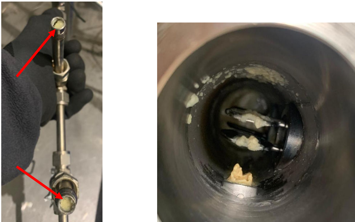
Figure 7: Pictures illustrating the white color of the wax found in the tubing at the outlet of the Fischer-Tropsch reactor (left) and brown color of the wax in the gas-liquid separator (right)..
