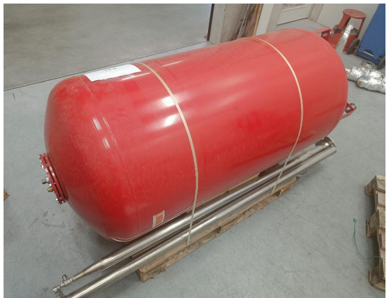
Figure 5: Low-pressure syngas buffer vessel of 800 L. The vessel is to be installed adjacent to the GtL system at the IMDEA site.
